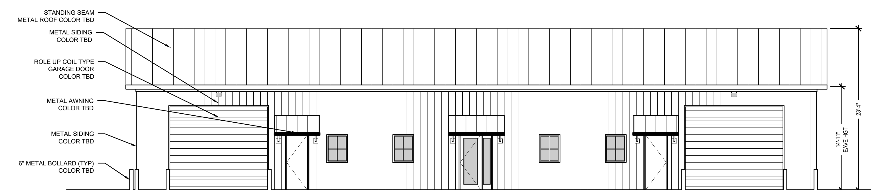
02 MAINTENANCE BUILDING - SOUTH ELEVATION SCALE: 1/8" = 1'-0"
