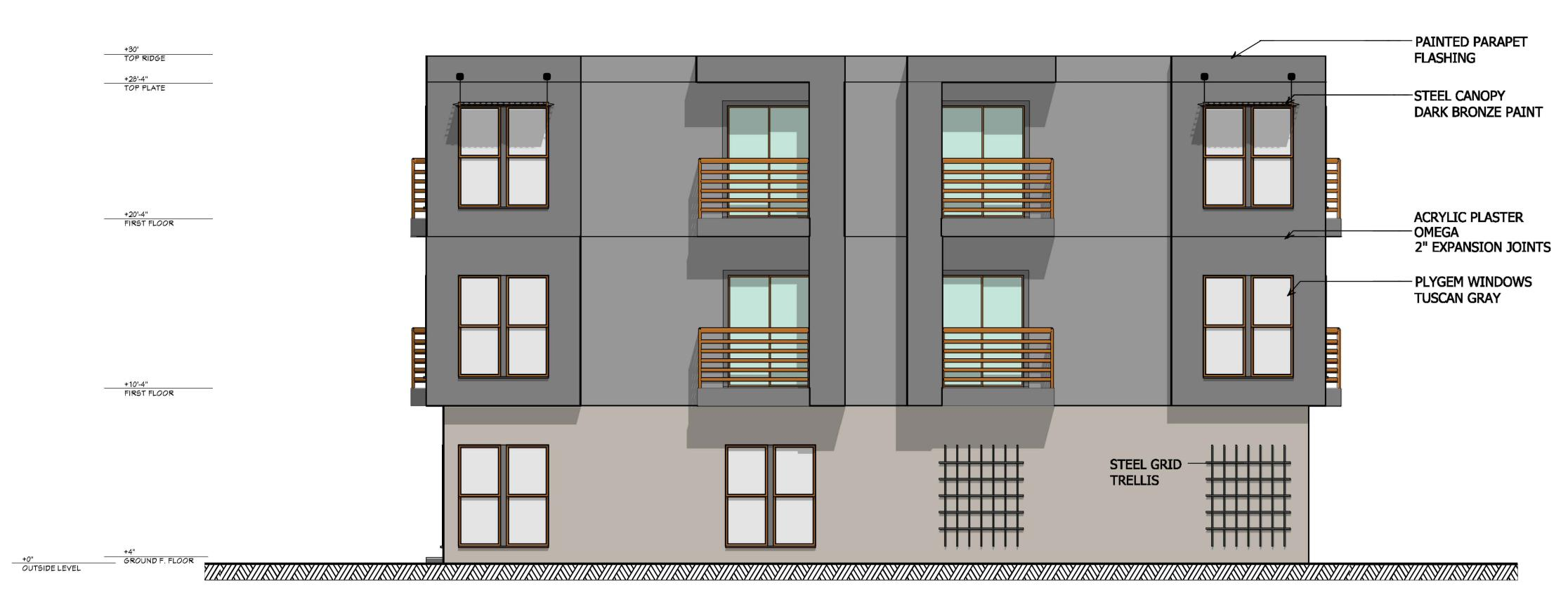
BLDG "C" NORTH ELEVATION SCALE: 1/4" = 1'=0"
