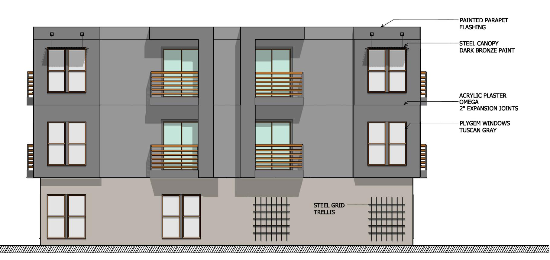
BLDG "B" EAST ELEVATION SCALE: 1/4" = 1'=0"
